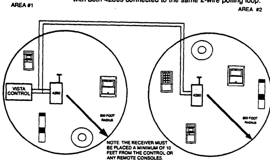
Diagram 12. TWO WIRELESS RECEIVERS TO INCREASE COVERAGE
