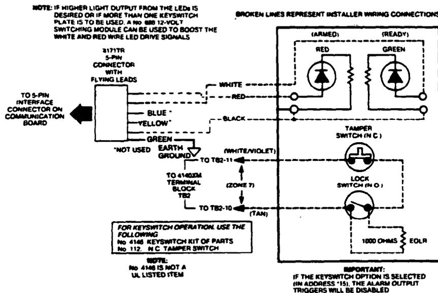
Diagram 30. KEYSWITCH WIRING
