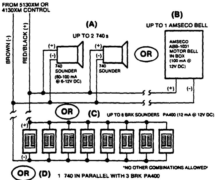
Diagram 16. SOUNDER OPTIONS FOR 5130XM OR 4130XM CONTROLS
